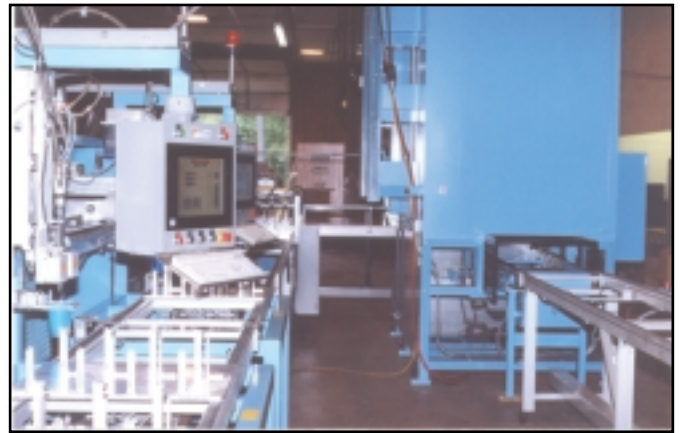
Conveyorized loop system. VertiCure™ vertical curing system at right; robots and robot touch-screens at left.
