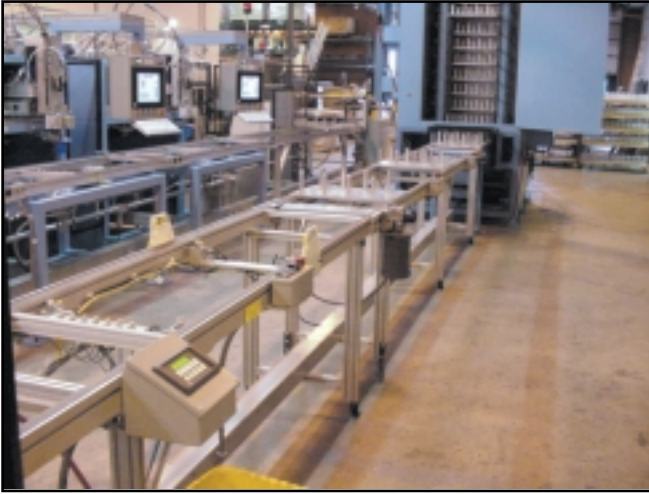
Part-style switching station at lower left. At upper right is the VertiCure™ door open to show series of pallets in cooling zone.
