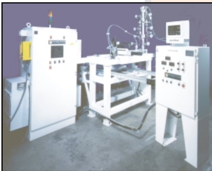
The Program-A-Spenser™ dispensing system (center), the main control enclosure (left), and the Program-A-Flow™ / Sense-A-Bead™ controls (right)
