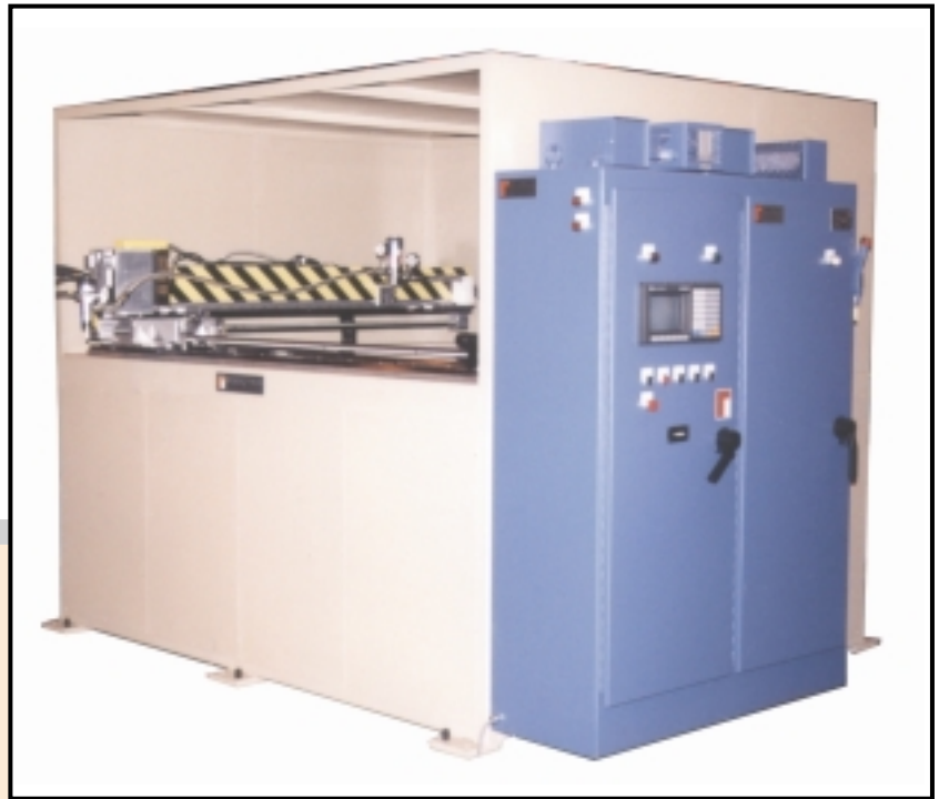
The HS Series Program-A-Spenser™ dispensing system. The headliners are automatically conveyed in front for dispensing, and are automatically conveyed out upon dispensing completion (existing production line not shown).
