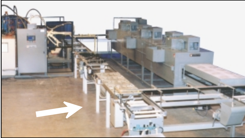
View of Cured-In-Place-Gasketing (CIPG) system. Operator load/unload station is indicated by arrow.
