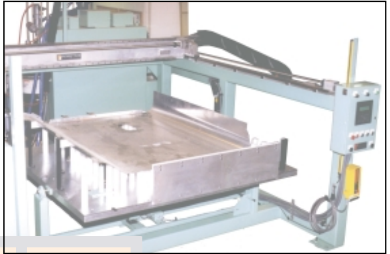
Cab body panel on the ergonomically-designed tilt-table fixture, ready for scuff and dispense. Teach pendant is below control panel shown at right.
