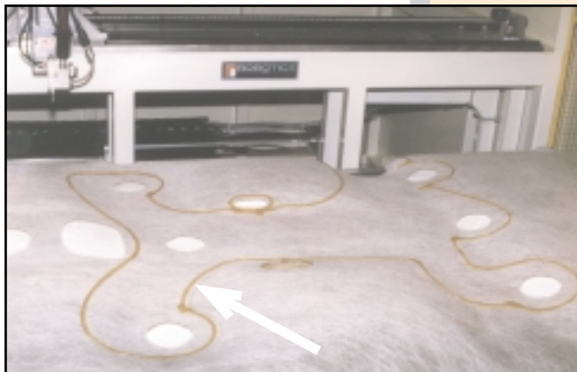
The adhesive bead outlining the aircap seal perimeter on the three-dimensional headliner surface.
