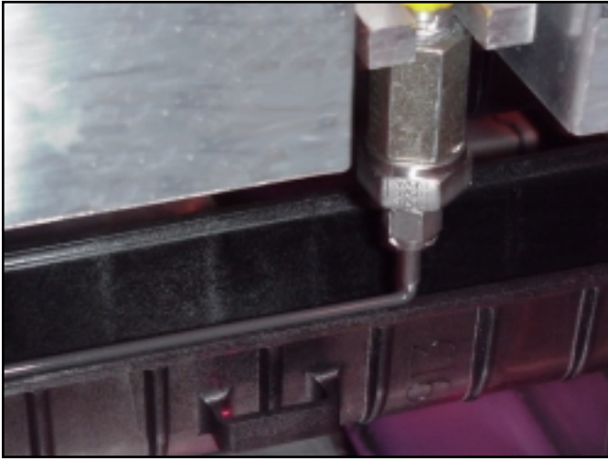
The bead of LSR is precisely applied at 400 inches per minute.
