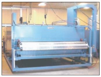
*Thermoforming Application* – The InfraCure<sup>TM</sup> 5000 rapidly brings a pair of 5' x 9' thermoplastic sheets to required temperature. The conveyor then automatically extends to present the heated sheets to the press. A height adjustment feature allows the oven to be raised or lowered to match the conveyor height with the press load height.
