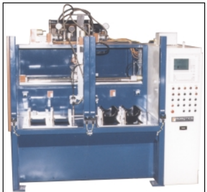
B Series dispensing system with left and right hand part fixture bays. Each bay holds two parts for dual-gun dispensing.
