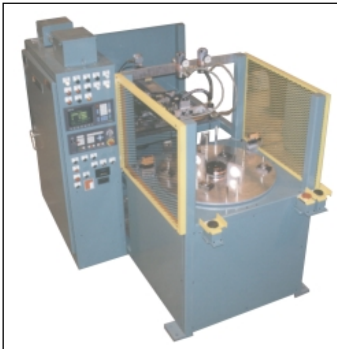
CR Program-A-Spenser™ automated dispensing system with a two-position dial table for increased production volume. Dial table includes adjustable pins for locating multiple parts.
